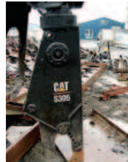
Caterpillar's S305 small mobile shear can run on a 7t excavator.
