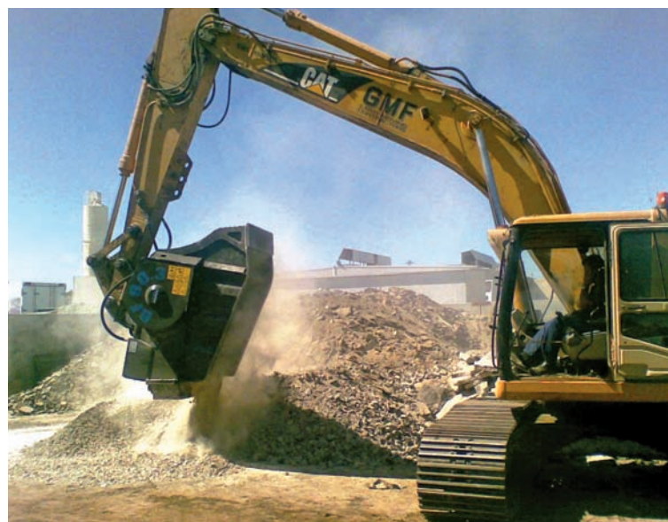
GMF Contractors' MB BF90.3 crusher bucket in action.
