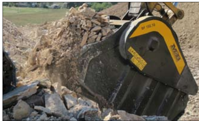
BF150.10, the biggest crusher bucket by MB
