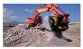
rushing in quarries around the world has become a key aspect of mines operation; the need to make the most of all available material arose and has prompted sharpest operators to use also the "waste material" that was once simply piled up in the quarry, becoming today valuable resources. The need remains to obtain the desired sizes in the shortest time possible maximizing the operating profitability per cubic meter worked as well.
