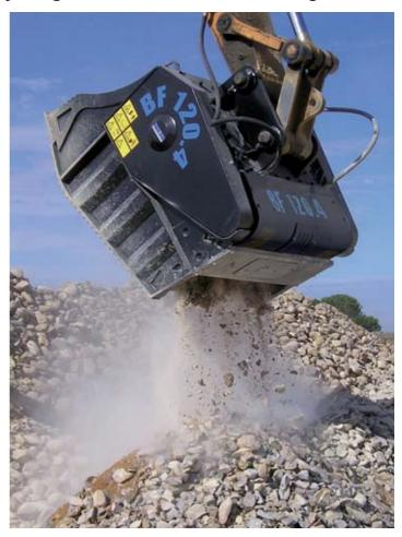
They visited the recycling site of their client, where demolition rubble from multiple sites together with excavation material and materials from natural rock quarries, are brought here for processing. The use of the bucket crusher has made the complete recovery of demolition material possible. For instance, this material, which was once taken to dumps, is extremely valuable in the road sector.
